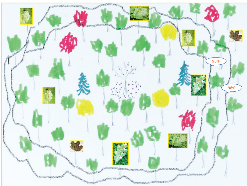
Sketch #1: This “Artist Rendering” of the DNR/Bruhn Model for Root Graft Disruption to stop Oak Wilt transmission through roots grafts involves placing two trench lines 5-6 feet deep around a large population of trees followed by destroying all oak trees within the trenches, including all healthy oak trees. This technique, needlessly destructive and promoted as the official recommendation by the Oak Wilt Coalition and an arborist society through the Oak Wilt Qualifications Program, cannot be consistent with Best Management Practices.
